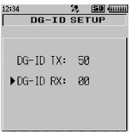
4 Press the key, then rotate the DIAL knob to set the receive DG-ID (DG-ID RX) to "50".
