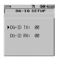
2 Press the [4] key, then rotate the DIAL knob to set the transmit DG-ID (DG-ID TX) to "50".
